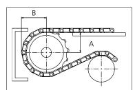
Other sprocket sizes are available upon request. Two-part sprockets are available upon request. Round bores are always delivered with keyway. Other bore sizes are available upon request. uni Retainer Rings: See uni Retainer Ring data sheet Width of single tooth = 10.0 mm (0.39 in) Width of sprocket = 50.0 mm (1.98 in)
