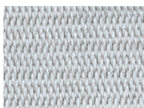
Broken twill weave GK Equally spaced air pockets
